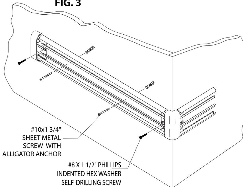
3. Drill marked holes on wall using a 1/4" drill bit and position Alligator anchors into holes. Mount retainer on wall and tighten screws to secure. Slide end caps and corners onto the retainer and secure, leaving a 1/16" gap between returns/corners and retainer to allow for adjustment. See Figure 3.
