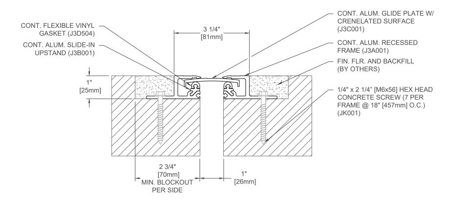
NOTE: TO DETERMINE BLOCKOUT DEPTH, DEDUCT THICKNESS OF THE FLOOR FINISH FROM FRAME HEIGHT
