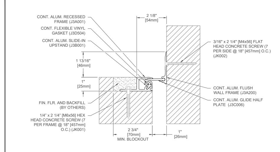
NOTE: TO DETERMINE BLOCKOUT DEPTH, DEDUCT THICKNESS OF THE FLOOR FINISH FROM FRAME HEIGHT
