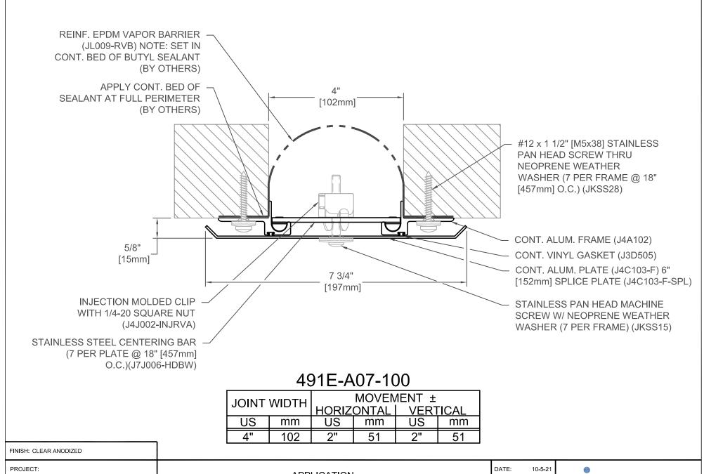
APPLICATION-EXTERIOR CENTERING BAR SYSTEM SURFACE MOUNT FRAME WALL/WALL, CEILING/CEILING CONDITION
