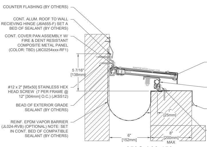
TELESCOPING ALUM SEISMIC ARMATURE w/ COMPRESSION SPRING FASTENING SYSTEM (PRE-INSTALLED)
