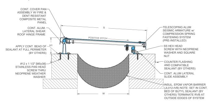
650C-A01-300 Roof/Roof With Fire Barrier (12" (305mm) system shown)
