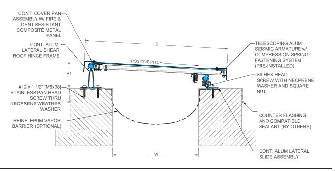
650C-A02-300 Roof/Wall (12" (305mm) system shown)
