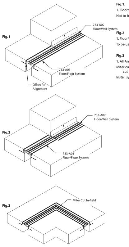
1. Floor/Floor system transitions to Floor/Wall (with alignment) Not to be used where fork lift traffic is present.
