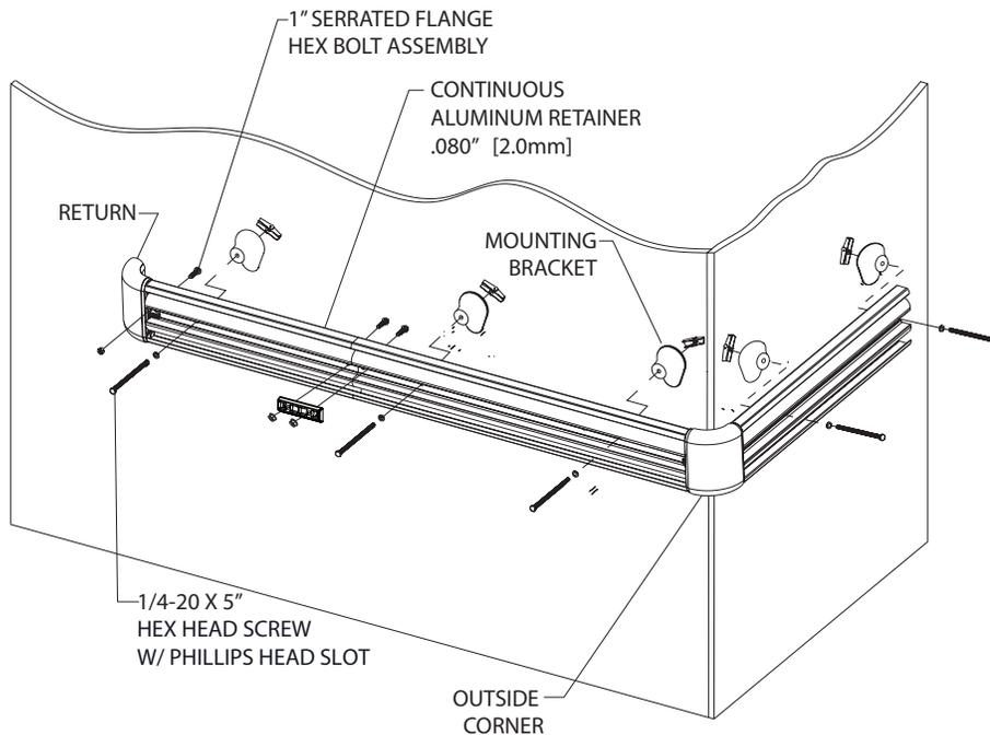
3. Attach returns and corners to retainer leaving a  $\frac{1}{16}$ " (1.5mm) gap between returns/ corners and retainer to allow for adjustment. Loosely attach brackets to retainer. Mount on wall, level retainer and tighten screws to secure. See Figure 3.
