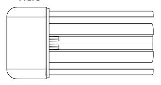
2. Attach Returns and Corners to retainer, leaving 1/16" gap between Return/Corner and retainer allowing for adjustment. **See Fig. 3**.
