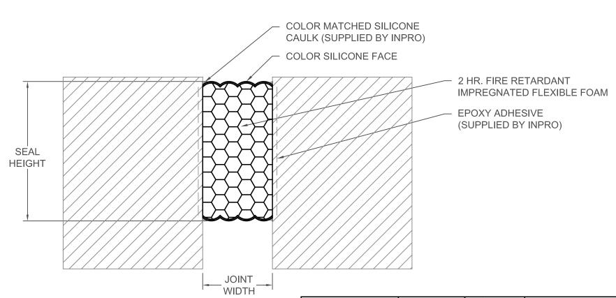
NOTE: SURROUNDING SUBSTRATE MUST MATCH OR EXCEED PERFORMANCE CAPABILITIES OF THE 990 FIRE RATED FOAM TO ACHIEVE FIRE RATING
