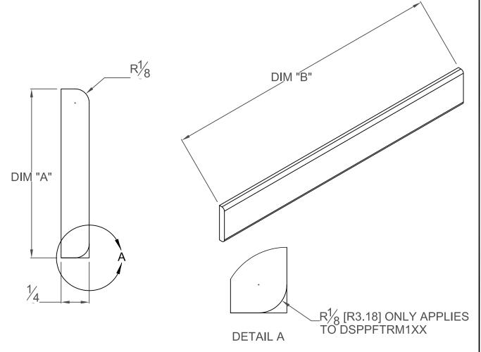
BOTTOM RADIUS ONLY APPLIES TO PARTS WITH DIM "A" OF 1.5" [38.1]
